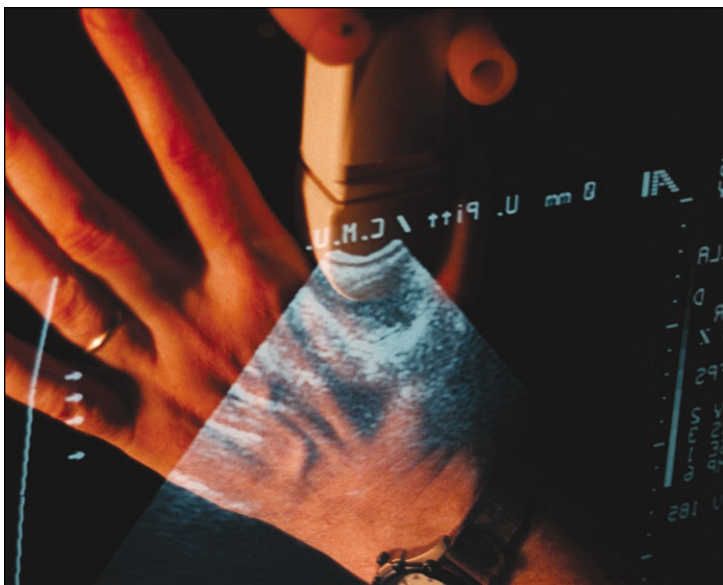
Figure 4. Photograph, from the viewpoint of the operator, showing a scan of a hand using the apparatus in Figure 2. The reflected ultrasonographic image is merged with the direct visual image.
