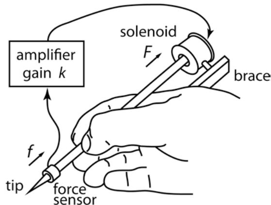
**Fig. 1** The Hand-Held Force Magnifier (HHFM) uses a sensor to measure force  $f$  between the handle and the tip, which is amplified to produce a force  $F = k f$  in the same direction on the handle using a solenoid mounted on the back of the hand.
