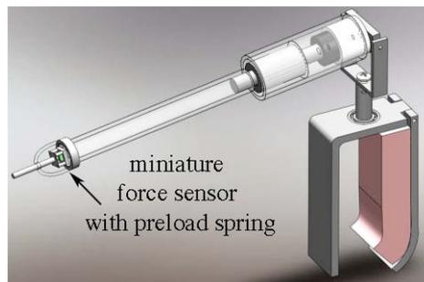
**Fig. 8** HHFM design with miniature distal force sensor.
