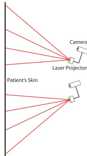
**Fig. 2** Structured light used to determine tilt of probe against skin.
