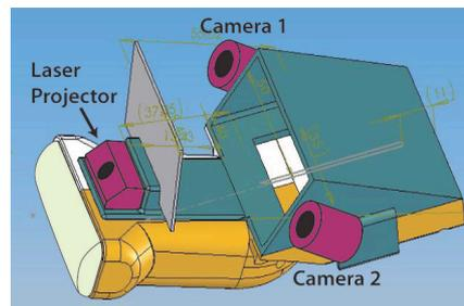
**Fig. 7** Plan for stereo cameras and a laser projector on the Sonic Flashlight.
