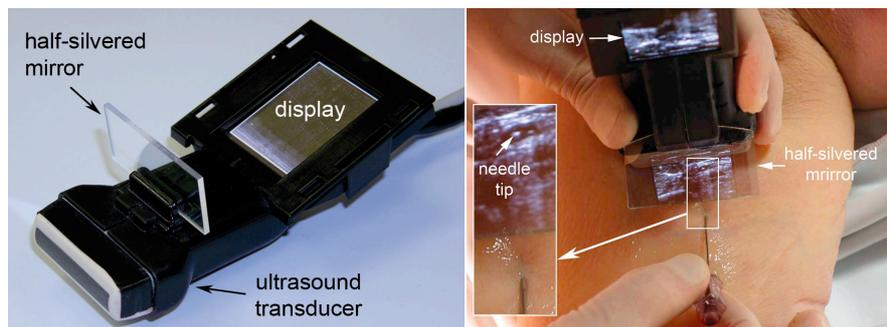
**Fig. 1** Sonic Flashlight device for viewing ultrasound in-situ (see text).
