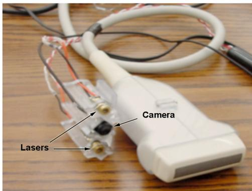
**Fig. 3** Design (top) and actual device (bottom) with camera and lasers mounted on probe.
