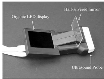
**FIGURE 1.** The Sonic Flashlight incorporates a Terason 10-MHz linear probe, a 54.8-mm organic light-emitting display, and a  $20 \times 50$ -mm 40% reflective mirror.
