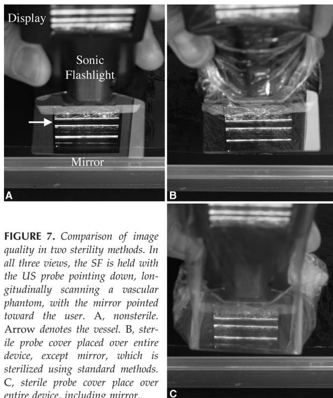
**FIGURE 7.** Comparison of image quality in two sterility methods. In all three views, the SF is held with the US probe pointing down, longitudinally scanning a vascular phantom, with the mirror pointed toward the user. A, nonsterile. Arrow denotes the vessel. B, sterile probe cover placed over entire device, except mirror, which is sterilized using standard methods. C, sterile probe cover placed over entire device, including mirror.
