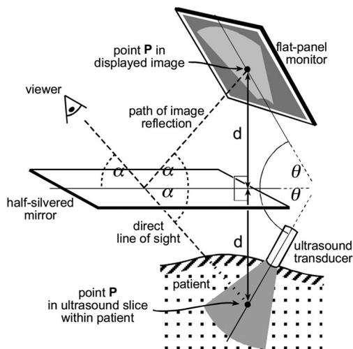
**FIGURE 2.** The half-silvered mirror bisects the angle between the US slice within the patient and the flat-panel monitor. Point P in the US slice and its corresponding location on the monitor are equidistant from the mirror along a line perpendicular to the mirror ( $d$ , distance). Because the angle of incidence equals the angle of reflectance ( $\alpha$ , angle), the viewer sees each point in the reflection precisely at its corresponding physical three-dimensional location.
