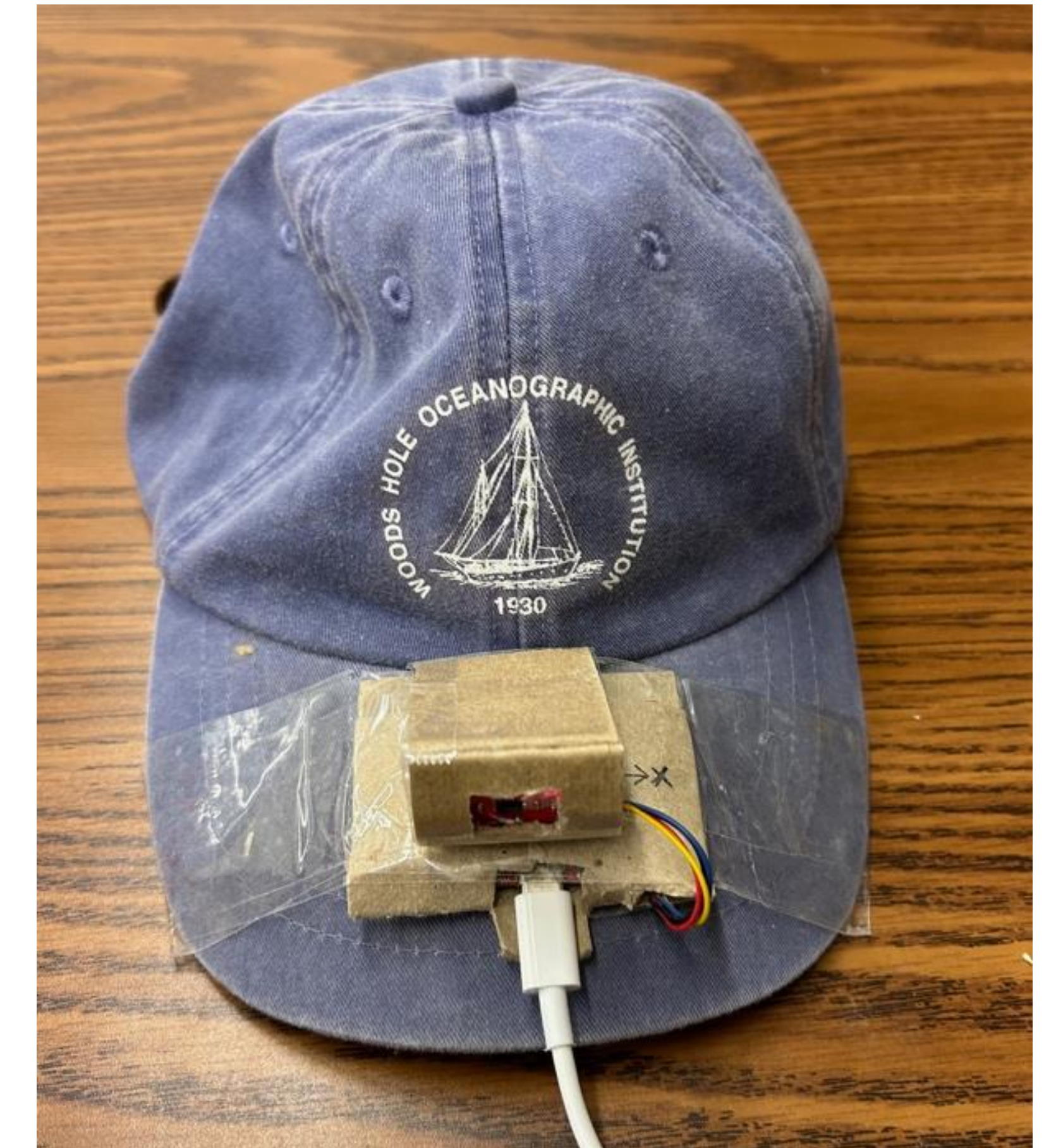
Figure A: SparkFun Data Logger affixed to cap for experimentation.
