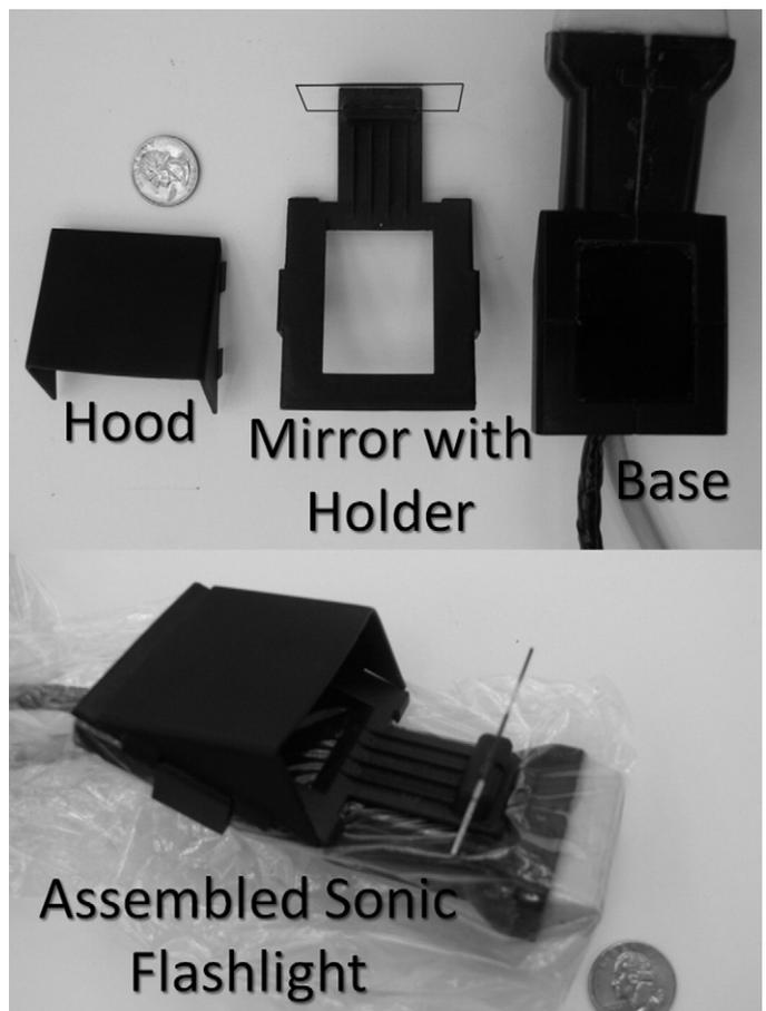
**Figure 4.** (Top) Revised version. The Sonic Flashlight, separated into three pieces, from left to right: hood, mirror with holder, and base. (Bottom) The assembled Sonic Flashlight with the plastic probe cover enveloping only the base.
