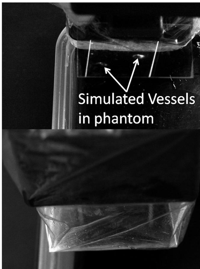
**Figure 3.** (Top) Initial version. Virtual image of two simulated vessels in a phantom seen through the half-silvered mirror with the plastic probe cover over the base only. (Bottom) The same virtual image seen through the half-silvered mirror with the plastic probe cover over the mirror. Note the degradation of image quality.
